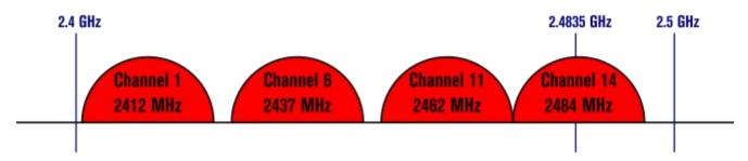
802.11g/n (OFDM) 20 MHz ch. width - 16.25 MHz used by sub-carriers
