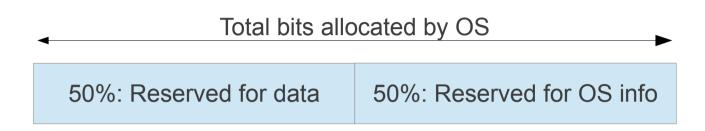
Of the memory allocated by the OS, assume half is for data received and half is for data structures used by the OS. What value should iperf server use for receiver window to achieve optimal TCP throughput?
