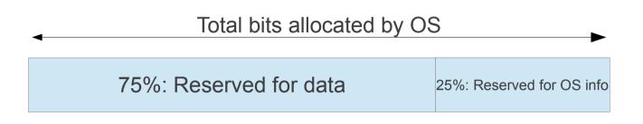
Of the memory allocated by the OS, assume 75% is for data received and 25% is for data structures used by the OS. What value should iperf server use for receiver window to achieve optimal TCP throughput?
