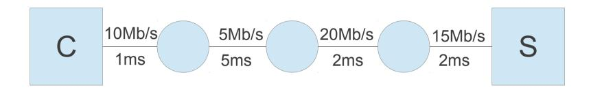
If UDP is used to send data from client to server, what is the maximum throughput that can be achieved? (ignoring header overheads)
