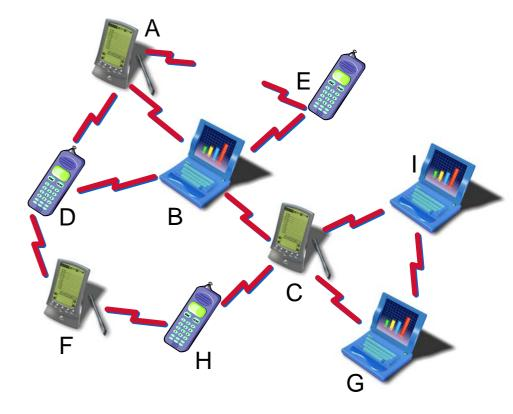
Called: ad hoc networks; mobile ad hoc networks (MANETs); wireless ad hoc networks; multi-hop wireless networks; ...
