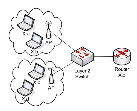
Notation: we will refer to IP addresses as *Network.Host* portion, e.g. *X.a* is an IP address on network *X* with host portion *a*
