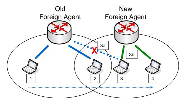
Connection with old FA is maintained for as long as possible, until it is no longer available (break, 3a); then connection with a new FA is established (make, 3b)
