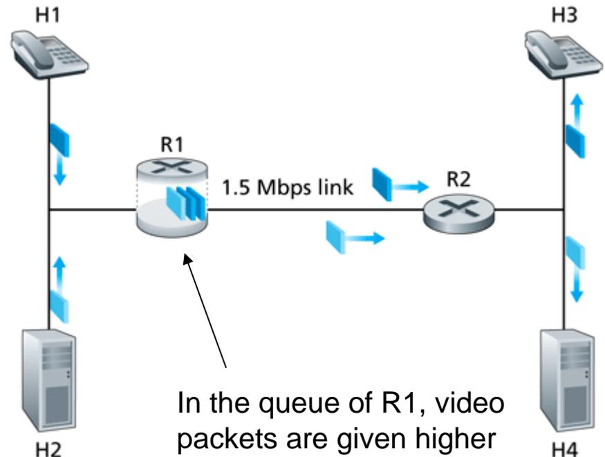
In the queue of R1, video packets are given higher priority than FTP packets
