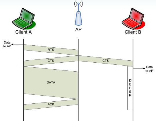
Using RTS/CTS before sending DATA reduces the probability of collision in the presence of hidden stations. When the AP responds with a CTS, Client B hears the CTS and immediately *defers* because someone else is about to transmit.
