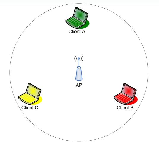
Lets assume all clients are within range of the AP, but no within range of any other client (e.g. A cannot hear B or C, B cannot hear C) All clients have data to transmit to the AP
