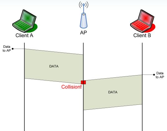
There is a high probability of collisions if using Basic Access in the presence of hidden stations. Client B starts transmitting because it believes the medium is idle (because Client B cannot hear Client A's transmission)
