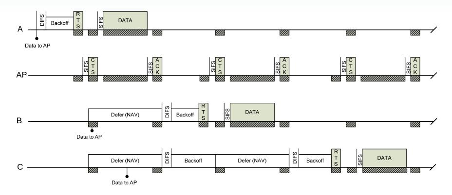
Even though the clients are hidden from each other, the use of the RTS/CTS means each client becomes aware of the other clients' transmissions (since each client hears the CTS from the AP). As a result there are no collisions: one station transmits at a time.
