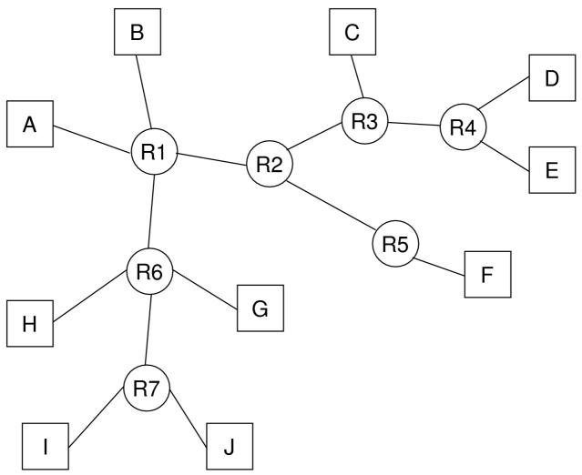
In the following cases, calculate the minimum number of packets that must be transmitted by the hosts and routers. For example, if host C sends a packet to host D, then the answer is 3: C transmits a packet to R3, R3 transmits a packet to R4 and R4 transmits a packet it D. State any assumptions if you make them.
