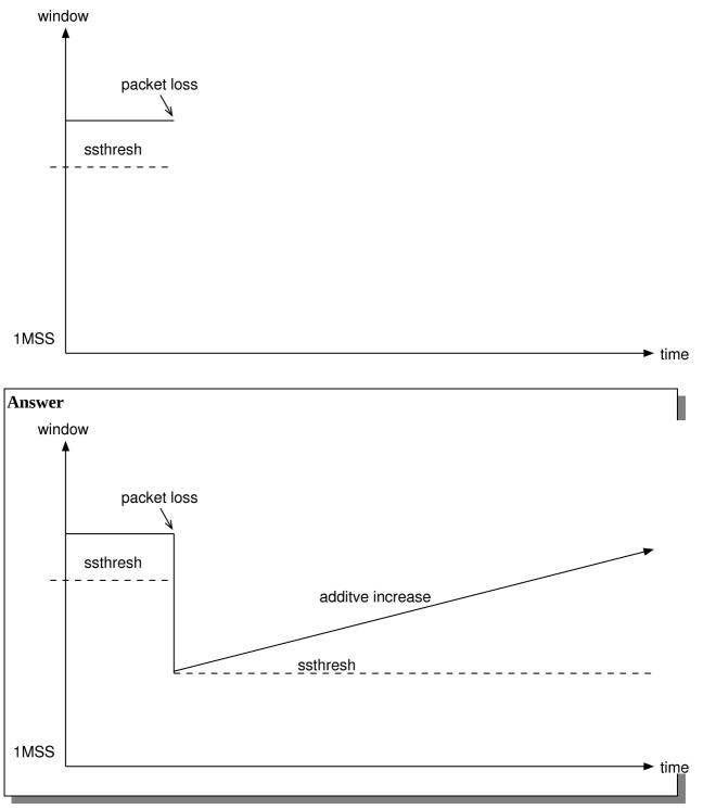
g) Explain why TCP source responds differently when there is a loss due to a timeout compared to when there is a loss due to a 3<sup>rd</sup> duplicate ACK. [3 mark]
