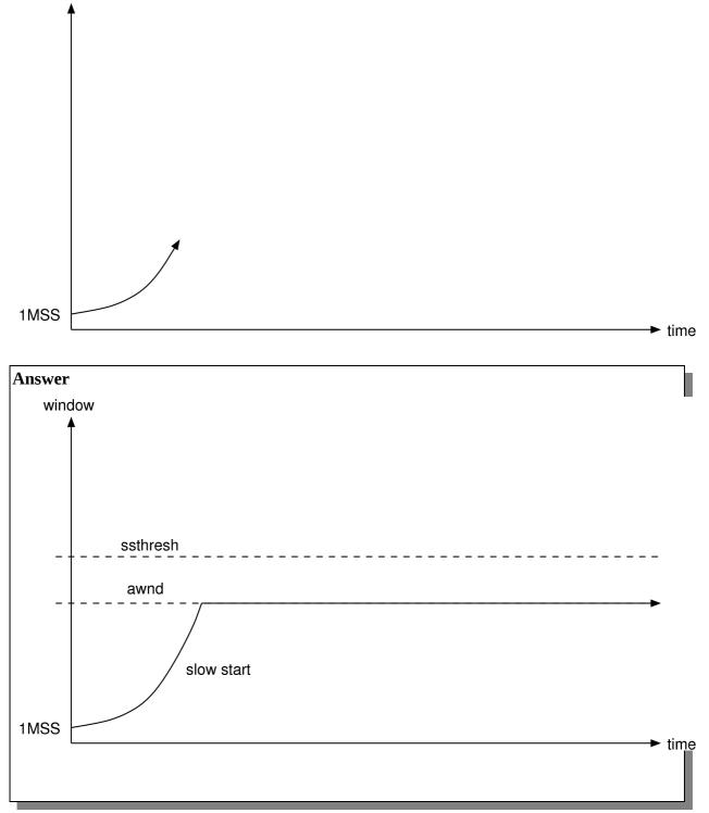
f) Buffer space at receiver is finite and greater than slow start threshold. Loss due to 3<sup>rd</sup> duplicate ACK occurs. Note that the diagram below shows the current value of the window when the loss occurs as a solid line. [3 marks]
