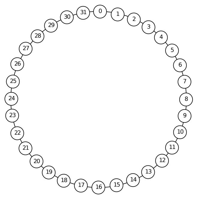
Assume currently the network contains 7 peers. The hash function H is used to determine the peer ID from the peers IP address and port number:
