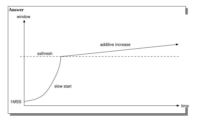
e) Buffer space at receiver is less than slow start threshold. No packet loss. [3 marks] window
