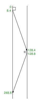
Propagation delay: 36,000 km @ 3x108 m/s = 120 ms
