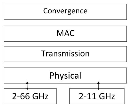
IEEE 802.16 Protocol Architecture has 4 layers: Convergence, MAC, Transmission and physical, which can be map to two OSI lowest layers: physical and data link.
