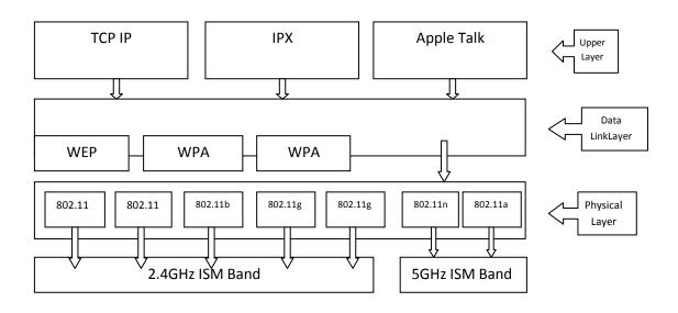
The Wireless Local Area Network (WLAN) technology is defined by the IEEE 802.11. There are currently four specifications: 802.11, 802.11a, 802.11b, and 802.11g. All four use the Ethernet protocol and CSMA/CA (carrier sense multiple access with collision avoidance instead of CSMA/CD) for path sharing.
