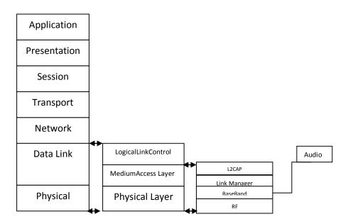
Bluetooth is defined as a layer protocol architecture consisting of core protocols, cable replacement protocols, telephony control protocols, and adopted protocols
