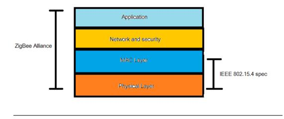
This picture, it shows the all the layers of ZigBee. Which contain four layers. There are Application, Network and security, MAC Layer and Physical Layer.
