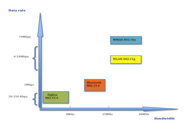
From this graph, you can see the efficiency of each technologies. In different technology, you can choose for specific task. For example Bluetooth we use on the mobile to send the small data and it is half duplex direction.
