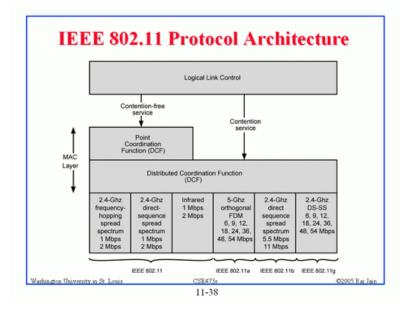
The 802.11 architecture is comprised of several components and services that interact to provide station mobility transparent to the higher layers of the network stack.
