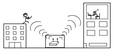
Ad Hoc Network It is decentralized wireless system. The temporary network is used; there are stations which provided the range into a temporary network. This is suitable for temporary linkage. For example, at Rangsit campus, a SIIT student's computer was use the Wireless LAN connection router to connect to another SIIT student's computer to transfer the files or the data to the destine (another computer).
