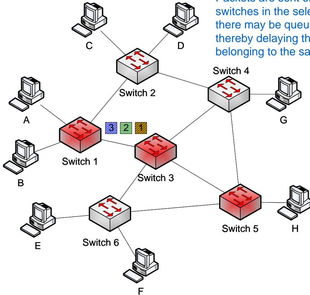
Packets are sent one at a time to the switches in the selected path. Note that there may be queuing delays in switches, thereby delaying the sending of Packets belonging to the same original data.
