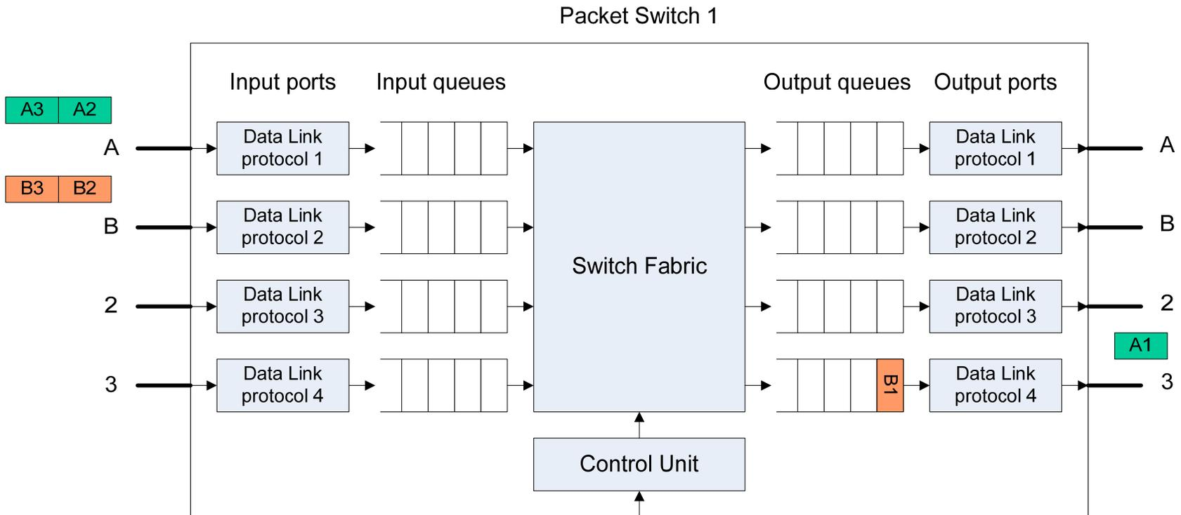
B1 must wait in the queue while A1 is transmitted. If output line rate is 1 packet per second, then B1 is in the queue for 1 second
