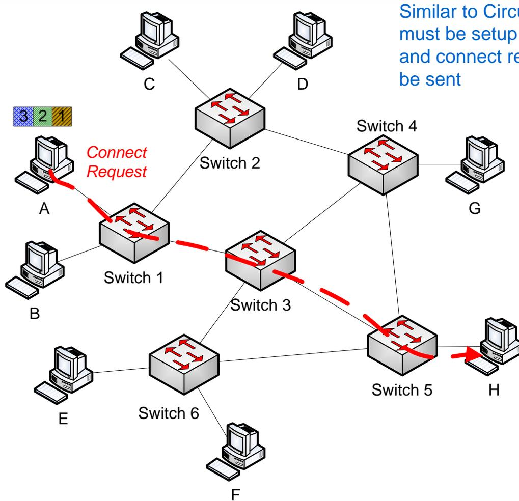
Similar to Circuit Switching, a connection must be setup (using connect request and connect response) before data can be sent
