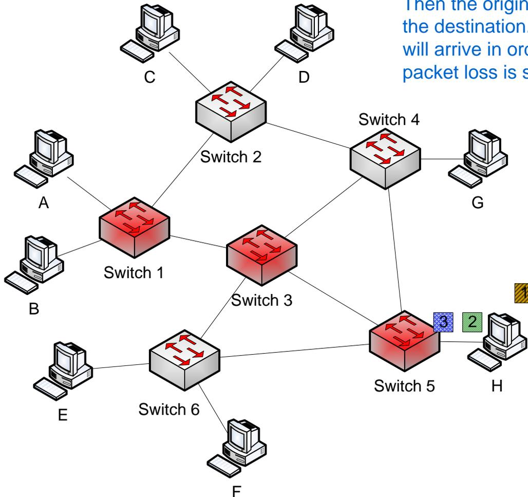
Then the original data is obtained at the destination. Note that the packets will arrive in order, although packet loss is still possible.
