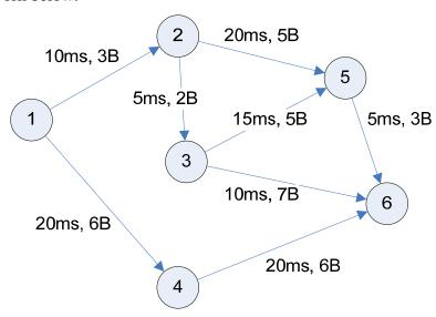
The delay (in milliseconds) and price (in Baht per MB) of each simplex link is shown. If a routing algorithm chose a path from 1 to 6 to be 1-4-6 then what metric was used by the least cost routing algorithm (select no more than one answer):
