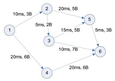
The delay (in milliseconds) and price (in Baht per MB) of each simplex link is shown. If a routing algorithm chose a path from 1 to 6 to be 1-2-5-6/1-2-3-6/1-4-6 then what metric was used by the least cost routing algorithm (select no more than one answer):
