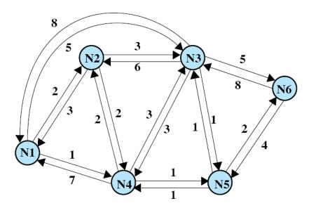
In the lecture, we calculated the shortest path tree from node N1. That is, the least-cost paths from N1 to N2, from N1 to N3, and so on. We used Dijkstra's algorithm to calculated these paths.
