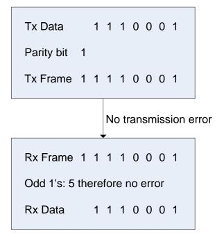
The parity check is successful: no error occurs, and no error is detected. The correct data is received.
