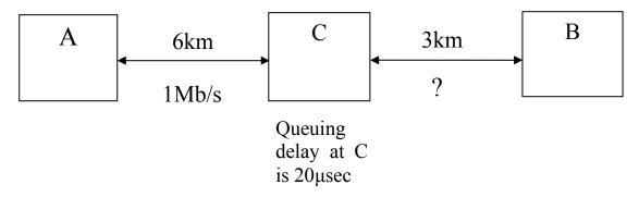
If a message of size 100 bits has to be sent from A to B with a maximum delay of 175/200/250usec, then
