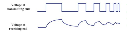
With attenuation and higher frequencies, it is harder to tell whether receiver signal is 0 or 1
