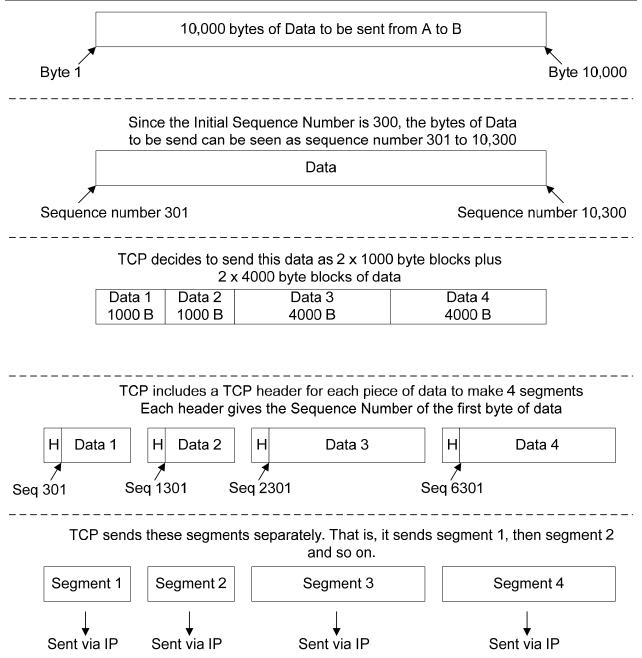
With Acknowledgments, the receiver indicates the *next byte expected to be received*. That is, when B acknowledges the first segment (which contain sequence number 301 to 1300 of data), then B includes an Acknowledgement Number of 1301.
