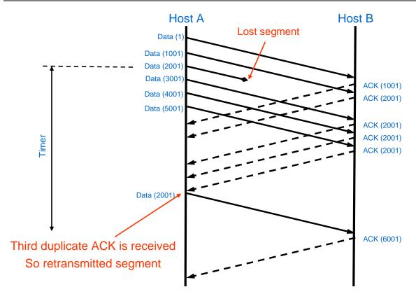
So using the same example as the Basic Retransmission scheme, when Host A receives the third duplicate ACK with Acknowledgement number 2001 (that is the fourth ACK(2001)), it assumes the segment with byte 2001 was lost and immediately retransmits. Host A will not wait for the timer to expire before retransmitting.
