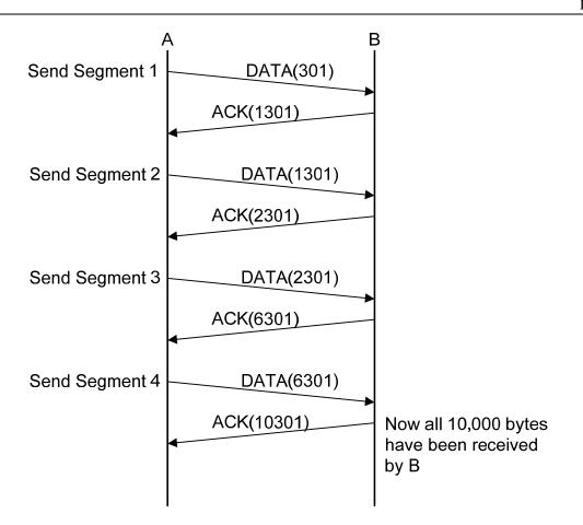
A similar process will be follow for B sending Data to A. In fact, B could send the Data with the ACKs.
