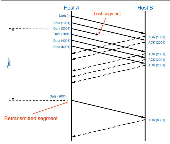
In this example, A has 6 segments to send to B, each of 1000 bytes. The Initial Sequence Number chosen by A was 0 (just for simplicity), and so the first sequence number is 1. The six segments are sent to B. Note that A does not wait for an ACK before sending all segments, we assume flow control allows A to send at least 6000 bytes at once.
