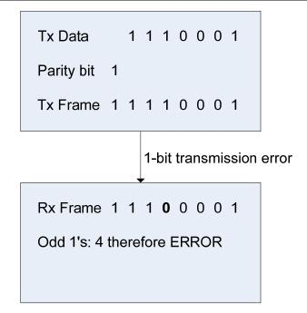
The parity check is successful: an error occurs, and the error is detected. The receiver does not receive the data (it will have to do something else in order to get the data, e.g. ask for a retransmission).
