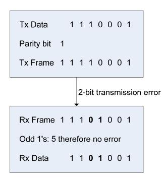
The parity check us **unsuccessful!** Errors occur, but the check does not detect these errors, and as a result the receiver receives incorrect data.
