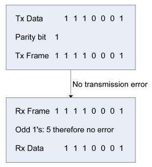
The parity check is successful: no error occurs, and no error is detected. The correct data is received.
