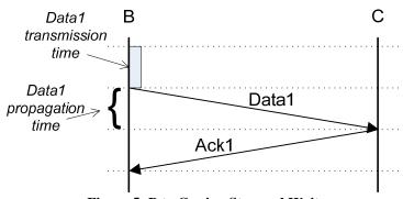
Figure 5: B to C using Stop and Wait
