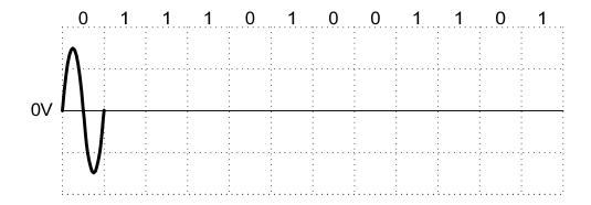
d) The bits are to be transmitted over an analog signal using a combination of Binary Amplitude Shift Keying and Binary Frequency Shift Keying. Complete the analog waveform below. [5 marks]
