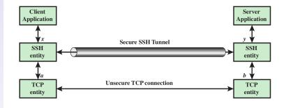
$\boldsymbol{x}$  and  $\boldsymbol{y}$  are application port numbers,  $\boldsymbol{a}$  and  $\boldsymbol{b}$  are port numbers used by SSH
