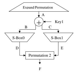
Expand/Permutation with 8 bit input, output bit order is: 4 1 2 3 2 3 4 1
