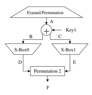
Expand/Permutation with 8 bit input, output bit order is: 4 1 2 3 2 3 4 1
