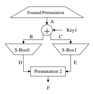
Expand/Permutation with 8 bit input, output bit order is: 4 1 2 3 2 3 4 1
