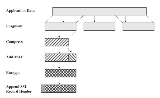
The figure below shows the steps applied to application data by the SSL Record Protocol.
