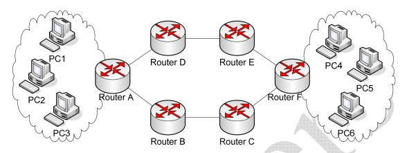
In parts (a), (b) and (c), assume IPsec with Encapsulating Security Payload and Transport Mode are used to secure data transfer between PC1 and PC4.
