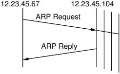
The ARP Request is broadcast whereas the Reply is unicast
