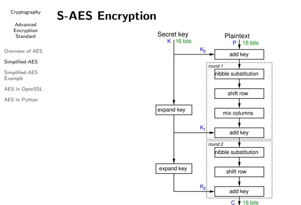
The figure on slide 9 shows the overall steps for S-AES and key expansion and encryption. The key generation takes a 16-bit secret key and expands that into 3 16-bit round keys. The first round key  $K_0$  is simple the original key. The next two round keys,  $K_1$  and  $K_2$  are generated by an expansion algorithm. The figure on slide 11 shows that algorithm for  $K_1$ .
