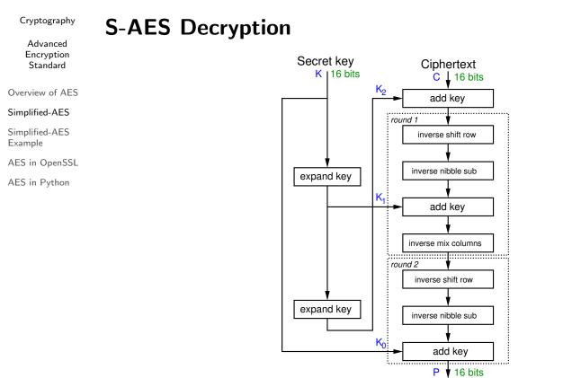
The figure on slide 10 shows the decryption operations. Note that it is similar to encryption in reverse, with all operations replaced with their inverse operations. The same round keys are used as in encryption, but in the opposite order.
