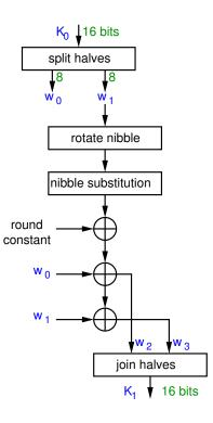
The figure on slide 11 shows the key generation operations for generated round key  $K_1$ . Similar steps are used to generate  $K_2$ , where the input is  $K_1$  and a different round constant.
