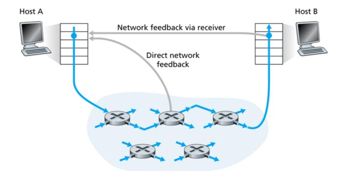
ATM is an example network technology using Network Assisted Congestion Control
