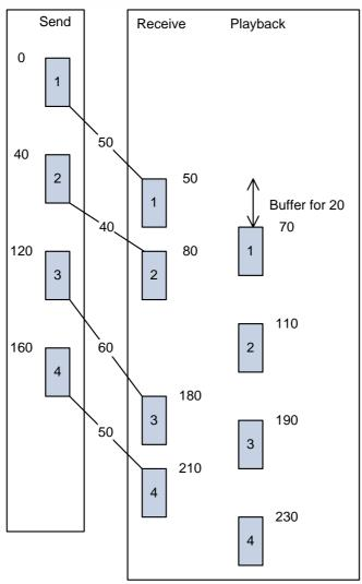
The receiver stores the each packet in a buffer (not played immediately).
