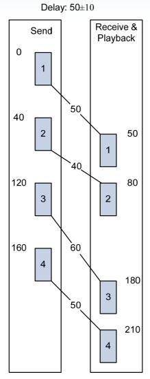
There is 50ms delay between when the source starts sending to when the playback starts at receiver.
