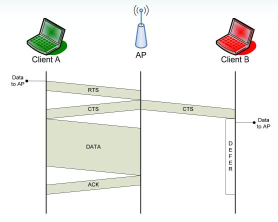
Using RTS/CTS before sending DATA reduces the probability of collision in the presence of hidden stations. When the AP responds with a CTS, Client B hears the CTS and immediately *defers* because someone else is about to transmit.
