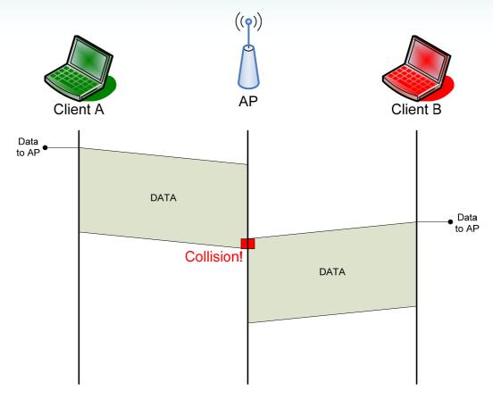
There is a high probability of collisions if using Basic Access in the presence of hidden stations. Client B starts transmitting because it believes the medium is idle (because Client B cannot hear Client A's transmission)
