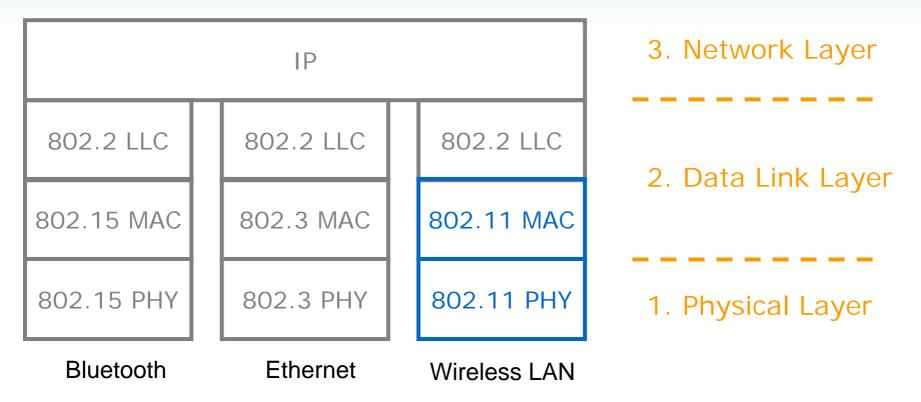
This shows an example set of stacks for a single laptop that supports wireless LAN, Ethernet and Bluetooth. Note that 802.2 is a common protocol for all 802 series LAN protocols. The MAC and PHY layers are specific to each LAN protocol
