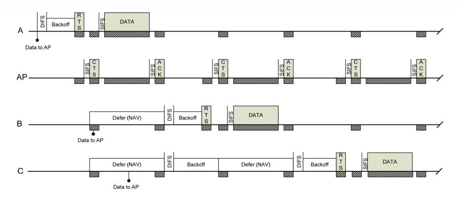
Even though the clients are hidden from each other, the use of the RTS/CTS means each client becomes aware of the other clients' transmissions (since each client hears the CTS from the AP). As a result there are no collisions; one station transmits at a time.
