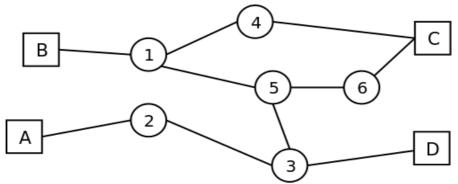
*Figure 2: Switching Network: Squares are stations; Circles are Switches*
