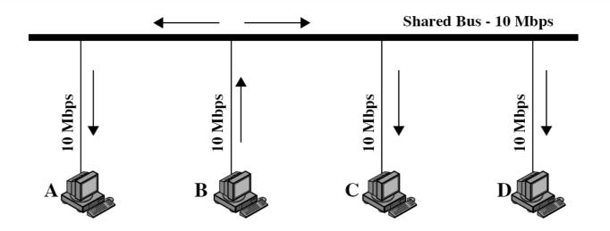
Ethernet in Bus Topology: only one station can transmit at a time (because a transmission goes everywhere on the bus) therefore stations must share the LAN capacity. Each station gets 2.5Mb/s
