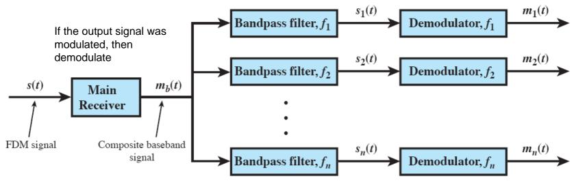
A bandpass filter only allows signal within a certain bandwidth to pass, thereby separating the output signal into individual user signals
