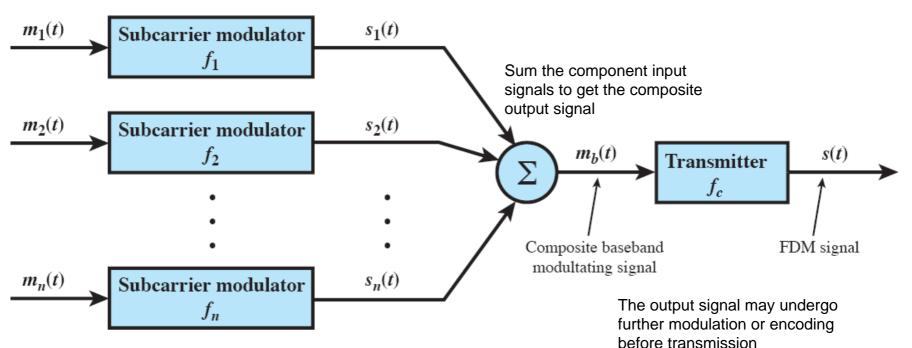
Modulate each signal onto a separate frequency (also remove components that are not necessary)
