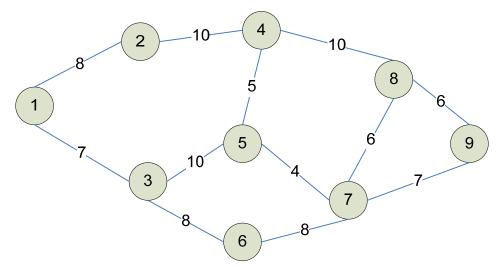
Now if the criteria for selecting a path (or route) is based entirely on the maximum capacity, then what path would be selected? In other words, what path should be based to allow for the highest amount of traffic to be sent from node 1 to node 9?
