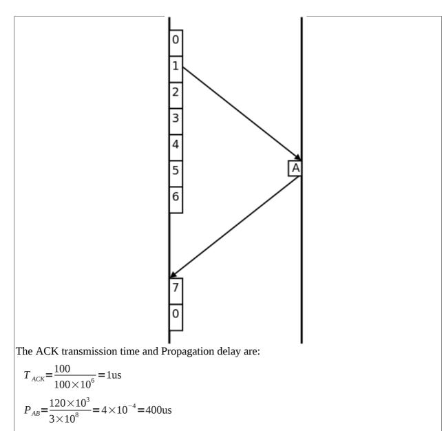
The time at which the ACK for the 1<sup>st</sup> DATA frame is received is: 901us
