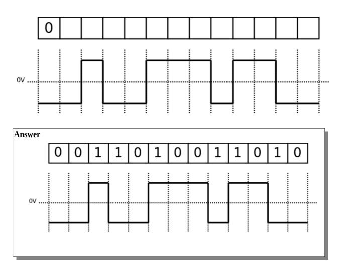
b) The Pseudoternary digital encoding scheme alternates between positive and negative voltage levels between successive bit 0's, and uses zero voltage for bit 1. Write the received bits in the boxes for the following received digital signal. [3 marks]
