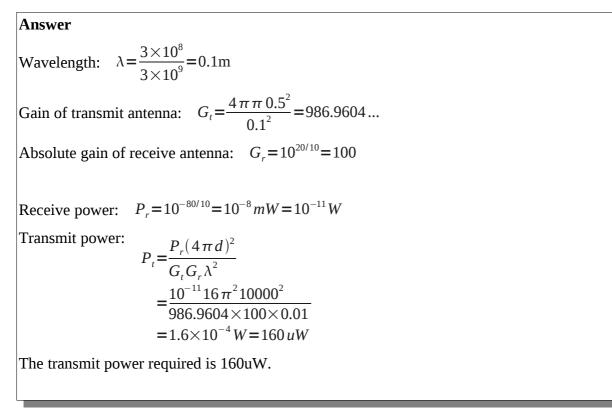
In the free space path loss model, the absolute path loss (L) between the two antenna's can be written as:
