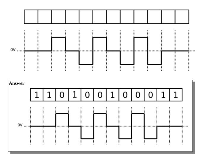
The following data is to be sent using a combination of FSK and ASK. There are 2 possible frequencies and 4 possible amplitudes.
