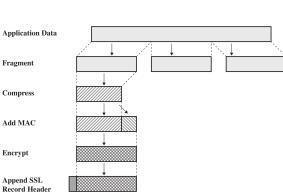
(b) Write an equation that expresses the SSL record operation on a single fragment, F from the client application that produces the packet to be sent P. Use the variables above and || for the concatenate/append operator. For function names you *must* use the algorithm names (i.e. you cannot use E() for encrypt, H() for hash; refer to specific algorithms). Denote the SSL header as SSL. [3 marks]
