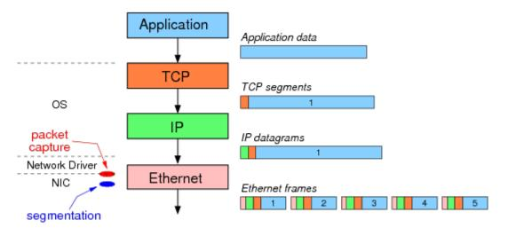
The result: although the same 5 Ethernet frames are sent over the network, Wireshark captures different data depending on the use of segmentation offloading. When not used, the 5 Ethernet frames are captured. When offloading is used, Wireshark only captures the single, large frame (containing 7,300 bytes of data).
